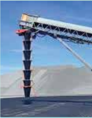
Telescopic chute for dust-free and controlled material loading.
