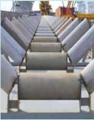
Conveyor idlers that reduce friction and maximize conveyor system life
