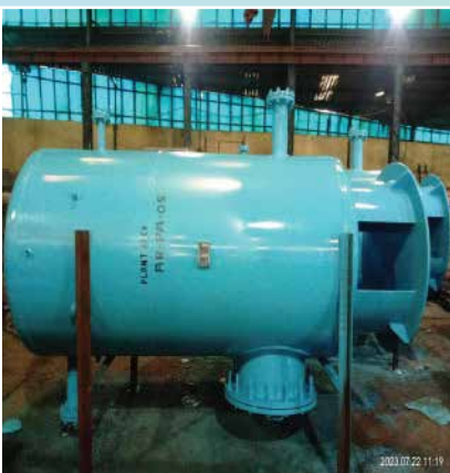
AIR RECEIVER (PLANT AREA)
